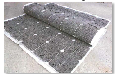
(Back-sheet after delamination)
